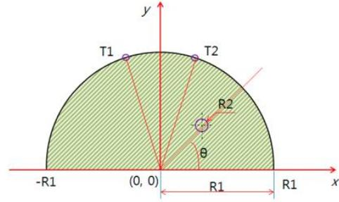
Figure 2: shows the thermal analysis model used in this study, where  $R1$  represents the left and right coordinates of both endpoints of the test model,  $R2$  represents the defect, and  $T1$  and  $T2$  represent the surrounding temperatures (Park and Yang, 2018).
