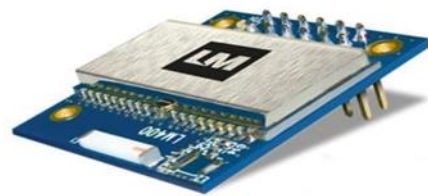
Fig 4: Bluetooth Module Onboard Antenna – LM400
