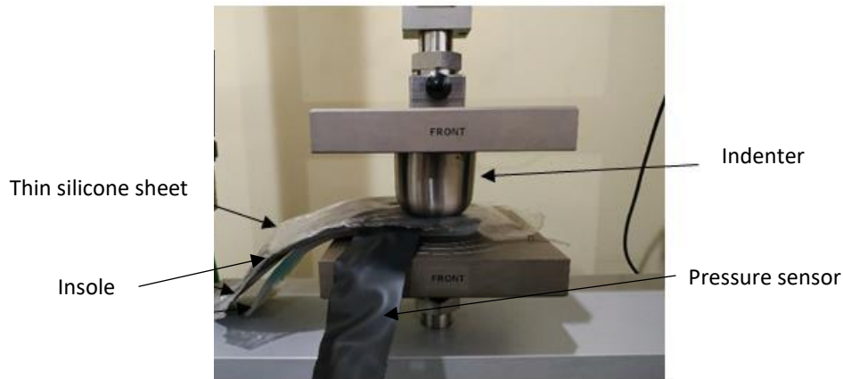
Figure 2: Test arrangement during testing with indenter and Tactilus pressure sensor
