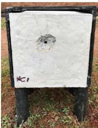
**Figure 4.5: Damage Pattern on the NC1 Block**
