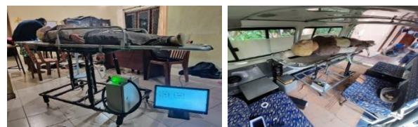
Figure 6. Final Fabricated Design of the Active Control Bed
