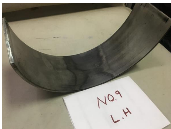
Figure 13. Metal wear down of No 09 bearing lower half
