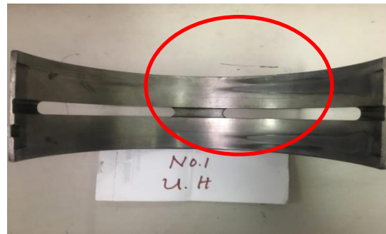
Figure 13. Metal wear down of No 01 bearing upper half
