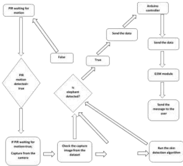
Figure 2. Flow chart of the existing Elephant detection system
