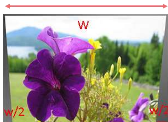
Figure 6: The trapezoidal image that is caused by the projector being elevated.
