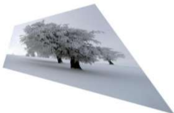
Figure 2: An oblique projector makes a bizarre trapezoid distorted display. An oblique projector makes a bizarre trapezoid distorted display.
